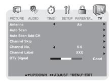
Antenna : Air (over-the-air broadcasts, Ch 2-69) or CATV (cable/satellite broadcasts, CH 1-135)
